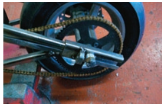
Chain tension and steel sleeves for brake calipers. me.
