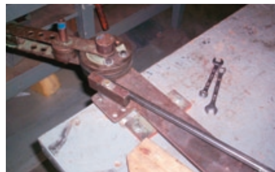
Steel formed in hydraulic pipe-bender.
