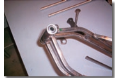
Headstock with golf kart bearing race inserted.
